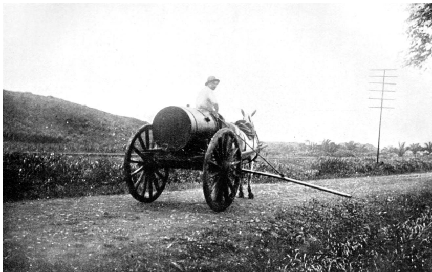
Figure 10.15 Oil cart designed to spray oil on the roadside ditches. This oil is controlled by a valve at the driver's hand. The pipe can be raised or made lower by a foot-pedal.
