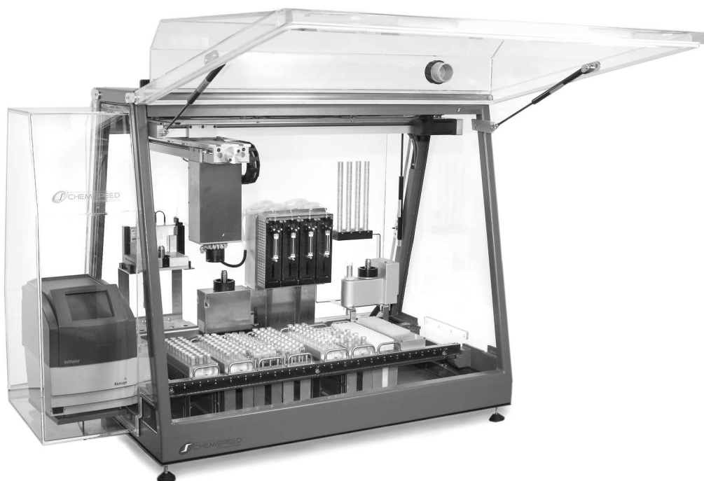
Figure 15.12 An example of an automated setup to robotically handle the microwave-catalyzed synthesis of numerous reactions and their subsequent automated purification. Shown here is a commercially available system, ChemSpeed SWave (ChemSpeed, Inc., Switzerland).
